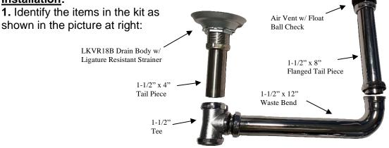
**2.** Install the drain body and 4" tail piece in the sink per the diagram from Elkay at right. Use putty or sealant.
