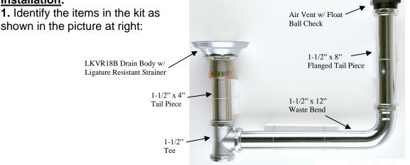
**2.** Install the drain body and 4" tail piece in the sink per the diagram from Elkay at right. Use putty or sealant.
