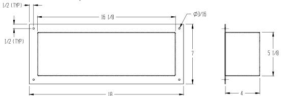
**3.** Verify that the recessed shelf cannot be loosened or removed. Fill any gaps between the wall and the flange with a security sealant (such as Pecora Dynapoxy EP-1200).
