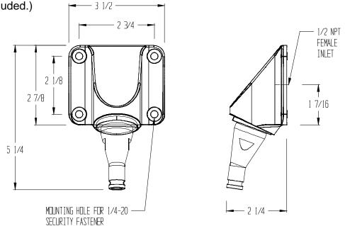
**2.** Verify that the SP-7WC cannot be loosened or removed. Fill any gaps between the wall and the tub filler with a security sealant (such as Pecora Dynapoxy EP-1200).
